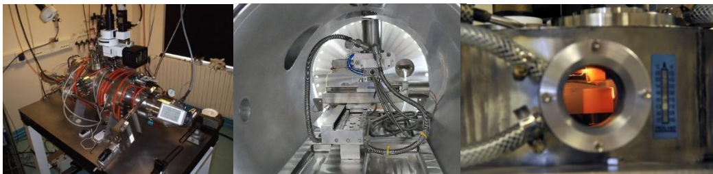
Figure 1. Hot hardness apparatus – Inside the vacuum chamber – sample and indenter furnaces –
